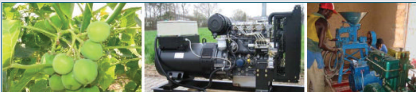
Fig. 3 - Jatropha Curcas (left) - the Africa's leader in biofuel race. Perkins engine (middle) with generator converted to run on Jatropha oil, is now installed in Kumasi, Ghana [6]. The Jatropha energy platform concept installed in villages in Mali - a multifunctional machine powered by Jatropha oil which combines generator, charger, oil press and mill [7]
