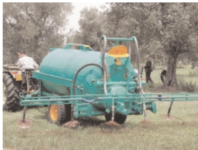
Figure 3 - Prototype of the waste water spreading machine
