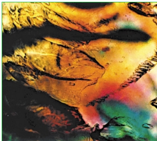
Figure 4 - Mesophasic behaviour of an HB aramide in NMP solution (ca. 60wt-%)
