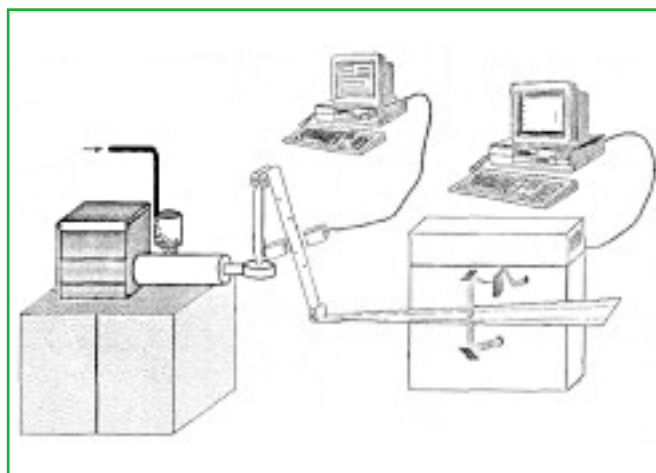
Figure 1 - Scheme of the apparatus consisting of: extruder, gel counter, FT-IR spectrophotometer
